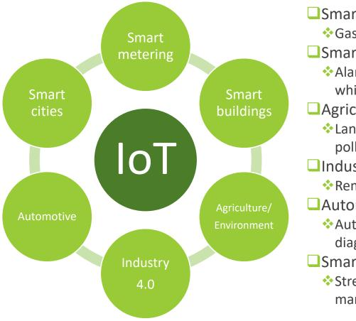
Smart metering ♦ Gas metering, water metering Smart buildings Alarm systems, HVAC, access control, white goods Agricultural/Environment Land/environment monitoring, pollution monitoring, animal tracking Industry 4.0 Remote control, asset tracking Automotive Autonomous driving, remote diagnostics Smart cities Streetlights, parking, waste management, ITS
