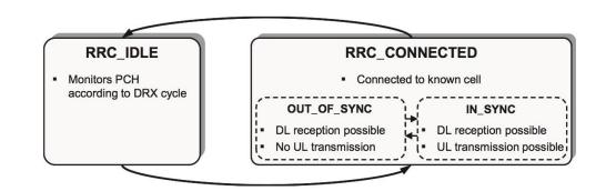
After transmitting a packet in uplink, the IoT terminal switches from RRC\_CONNECTED to RRC\_IDLE, losing the synchronization with the eNB and generating a lot of signaling to re-establish the connection.
