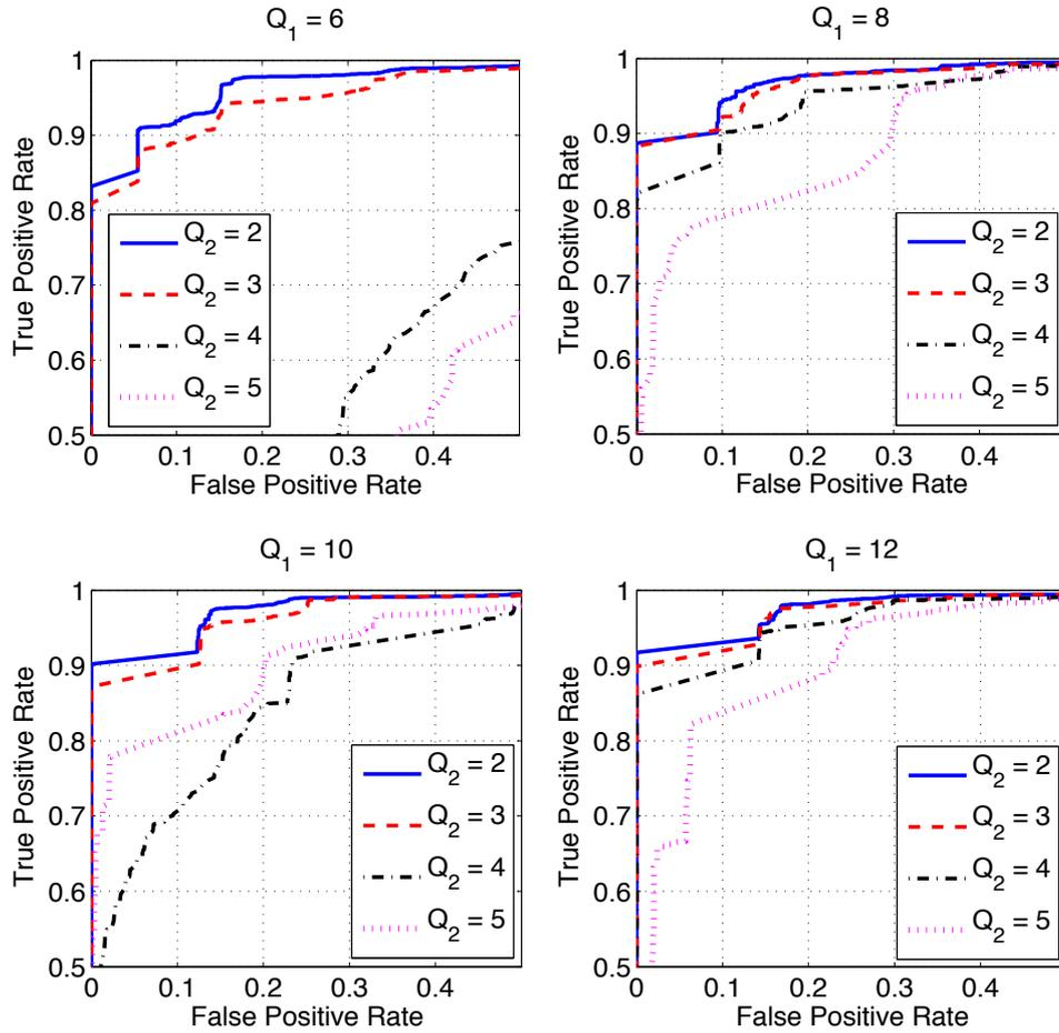
**Figure 6.15:** ROC curves obtained for the examined combination of  $Q_1$  and  $Q_2$ . From top left to bottom right, increasing values of  $Q_1$  are considered, and performance for varying values of  $Q_2$  are plotted (notice that curves have been magnified to improve readability). As expected, lower values for the second compression facilitate the localization.
