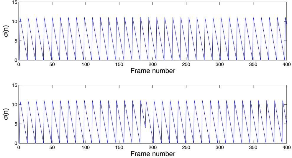
**Figure 6.5:** An example of the shift signal  $\sigma(n)$  for a double compressed sequence (top) and a manipulated sequence (bottom).
