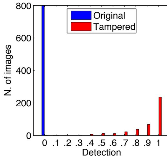
**Figure 3.3:** Histogram of outputs obtained by running the forensic tool in [35] on a set of images, some of which containing the forensic trace searched by the tool and some not. Red bars represent the outputs obtained on images containing the trace.
