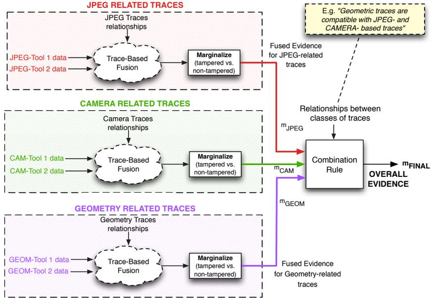
**Figure 3.2:** Block diagram illustrating the proposed approach to hierarchical fusion of traces of different kind. The “Trace-Based Fusion” bubble represents the schema in Figure 3.1.
