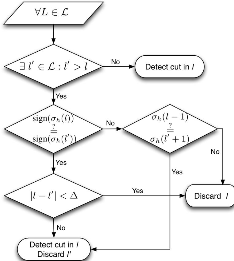
**Figure 6.6:** Algorithm for cut detection, given the set of indices where the signal  $\sigma'_h(n)$  is not null.
