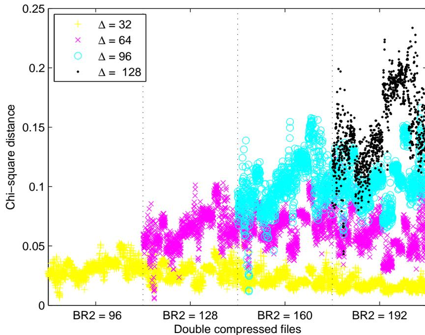
**Figure 10.3:** Chi-square distances computed for double compressed files with positive  $\Delta$ , grouped according to both the values assumed by  $\Delta$  and BR2.
