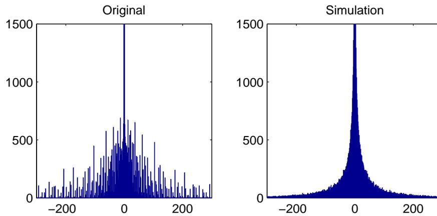
**Figure 9.1:** Histograms of MDCT coefficients of an MP3 file double compressed at 64 kbit/s and then 160 kbit/s (left), and of the corresponding calibrated signal at 160 kbit/s (right).
