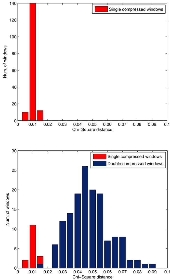
**Figure 9.6:** Histogram of  $D_\chi$  values on two analyzed audio tracks: (a) genuine audio track; (b) tampered audio track. The different colors highlight the two Gaussian components found by the EM algorithm.
