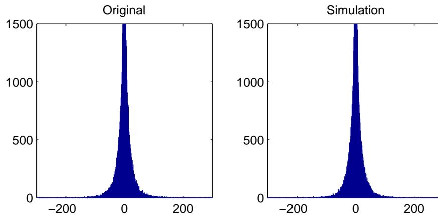
**Figure 9.2:** Histograms of MDCT coefficients of an MP3 file single compressed at 160 kb/s (left), and of the calibrated signal at 160 kbit/s (right).
