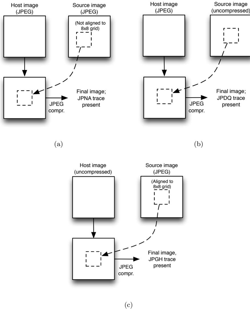
**Figure 4.1:** In these schemes three different configurations of cut&paste attacks are reported. The attack in (a) introduces a misaligned double compression, the one in (b) introduces the double quantization effect in the untouched part of the final image and the attack in (c) introduces the ghost effect in the pasted region.
