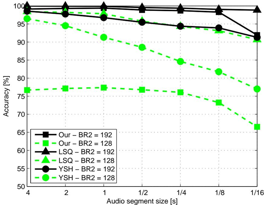
**Figure 10.4:** Detection accuracy with varying audio file duration for BR2=192 kbit/s and BR2=128 kbit/s.
