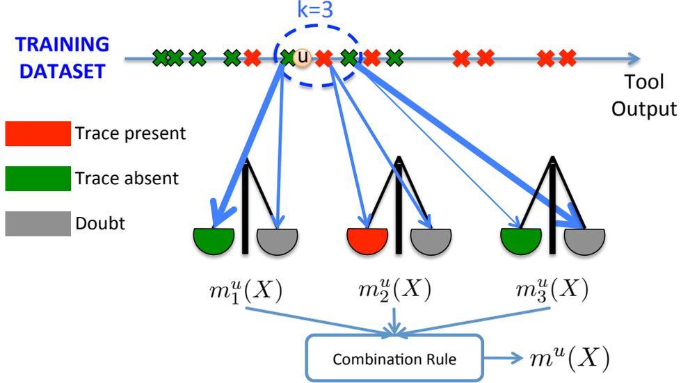
**Figure 3.5:** Graphic representation of the proposed method for mapping tool outputs to BBAs. The weight of each arrow connecting the unseen sample  $u$  one side of the balances model the amount of mass assigned to the corresponding proposition. As we can see, the farther the training sample is from  $u$ , the more mass goes to doubt.
