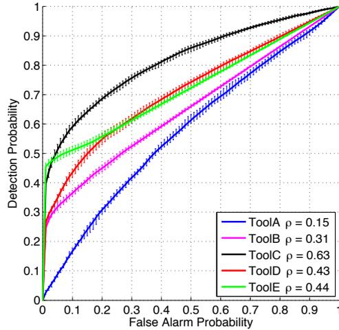
**Figure 4.5:** Performance obtained by each forensic tool alone on the synthetic test dataset. Although tools do not require a training phase, uncertainty bars are reported because their evaluation is repeated on different selections of the test dataset.
