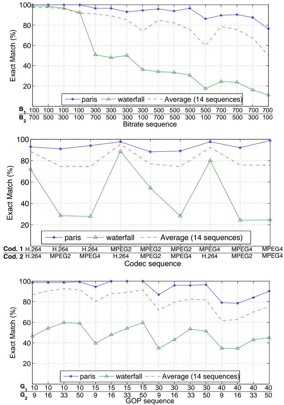
Figure 6.4: Performance of the method as a function of the  $B_1$ - $B_2$  bitrate (top), of the codec combination (middle), and of the  $G_1$  -  $G_2$  combination (bottom).
