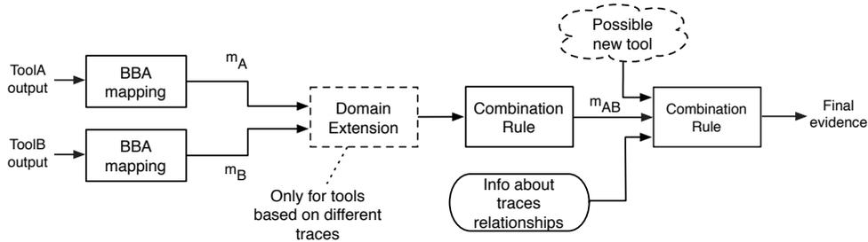
**Figure 3.1:** Block diagram of the proposed fusion approach. Notice that, when a new tool becomes available (represented in the dashed cloud), its BBA directly enters the final stage of the fusion, without the need to recombine information from previous tools.
