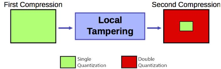
**Figure 6.8:** Idea underlying DQ-based forgery localization: pixels that do not expose traces of double quantization are considered as tampered.
