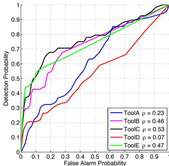
**Figure 4.8:** Performance obtained by each forensic tool alone on the realistic test dataset. Differently from Figure 4.5, uncertainty bars are not present because the whole realistic dataset is always used as the test set.
