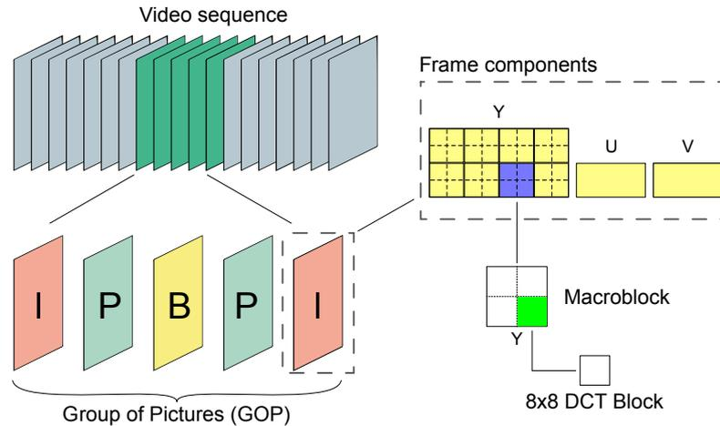
**Figure 5.1:** Structural elements in common video coding schemes.
