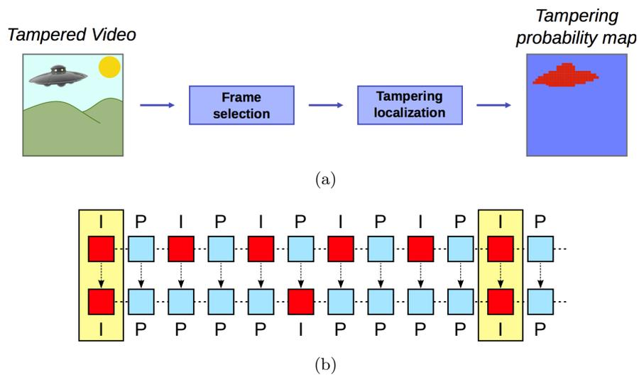
**Figure 6.7:** Schematic representation of the proposed approach: a subset of the frames is selected, then tampering localization is carried separately on each frame to obtain a forgery map (a). Specifically, those frames that have been intra-coded twice are selected (b).
