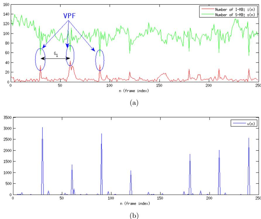
**Figure 6.2:** (VPF analysis carried on a double encoded video, with  $G_1 = 30$  and  $G_2 = 50$ : in (a) the number of I-MBs and S-MBs as a function of the frame number is plotted, while (b) shows the derived strength signal, obtained according to equations (6.1) and (6.2).
