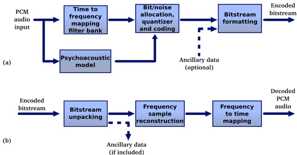
Figure 8.1: High level block diagram of MP3 coding (a) and decoding (b).
