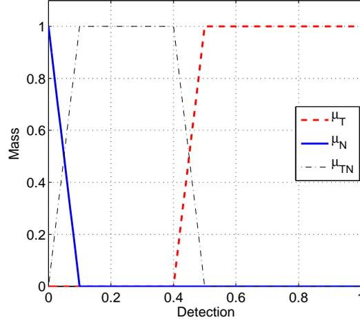
**Figure 3.4:** A possible way of defining output mapping functions for the forensic tool in [35].
