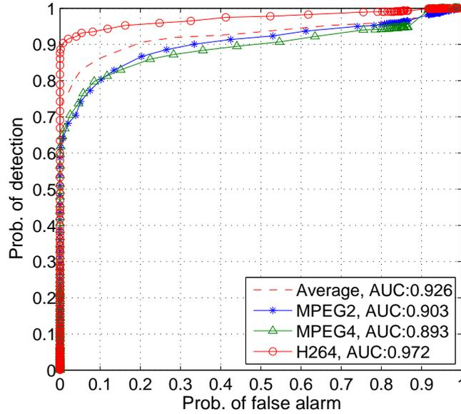
Figure 6.3: ROC curve for the proposed double encoding detector.
