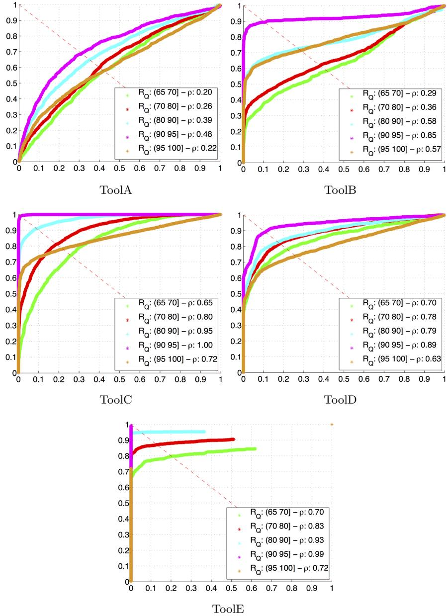
**Figure 4.4:** ROC curves for tools in  $\mathcal{F}$  for different ranges of last JPEG compression quality factor:  $\mathcal{R}_Q(a, b]$  denotes the set of all images in the dataset whose last compression quality factor falls within  $(a, b]$ . In each plot, the probability of detection  $P_D^f$  is plotted against the probability of false alarm  $P_{FA}^f$ .
