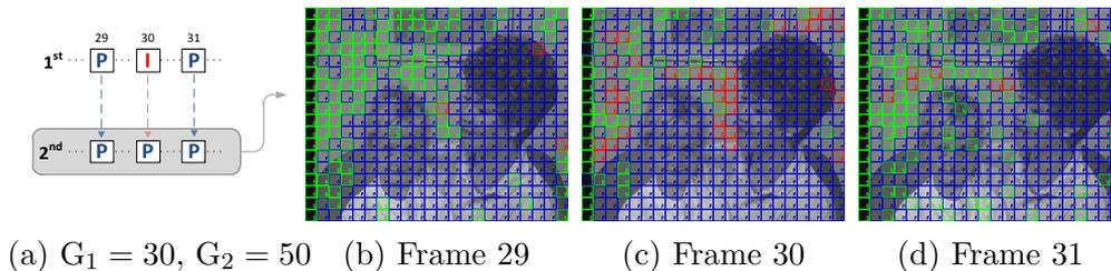
**Figure 6.1:** Example where the VPF is present in frame 30. Leftmost picture shows the types of frames with indices 29, 30 and 31 for both compressions. The remaining three pictures represent the macroblock types for each frame. Red color is used for I-MB, blue color for P-MB and green color for S-MB. Both first and second encodings are carried out using the x264 library, with a QP fixed to 20.
