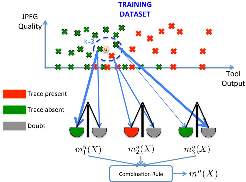
**Figure 3.6:** Graphic representation of the proposed way to include background information in tool output interpretation. In this example, only one image property is considered (the JPEG quality factor) for clarity.
