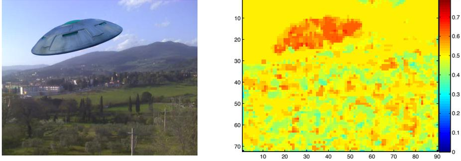
**Figure 6.13:** An intra-frame tampering (left figure) and the produced probability map (right figure). For showing purposes, a  $3 \times 3$  median filter has been applied to the map.
