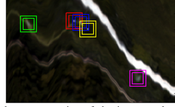
Fig. 1. True-color representation of the image analyzed. An EW is superimposed over each target. Targets enclosed by red, blue, and yellow EWs are contaminated by the presence of targets of the same type in their surroundings. The target encircled by the pink EW is placed in a non-homogeneous local background.
