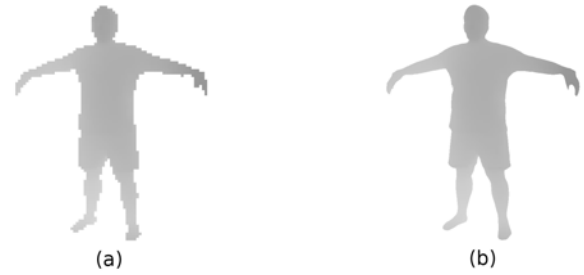
Fig. 13. Depth maps' comparison - (a) initial depth map; (b) output depth map.
